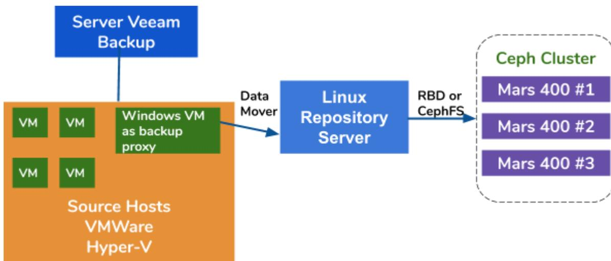
There are three ways to use the Ambedded Ceph appliance as the repositories for Veeam Backup and Replication. [CephFS](#) and [RBD block devices](#) can be used as the on-premises backup repository. The [S3 object storage](#) can be used as the capacity tier for a remote location.
